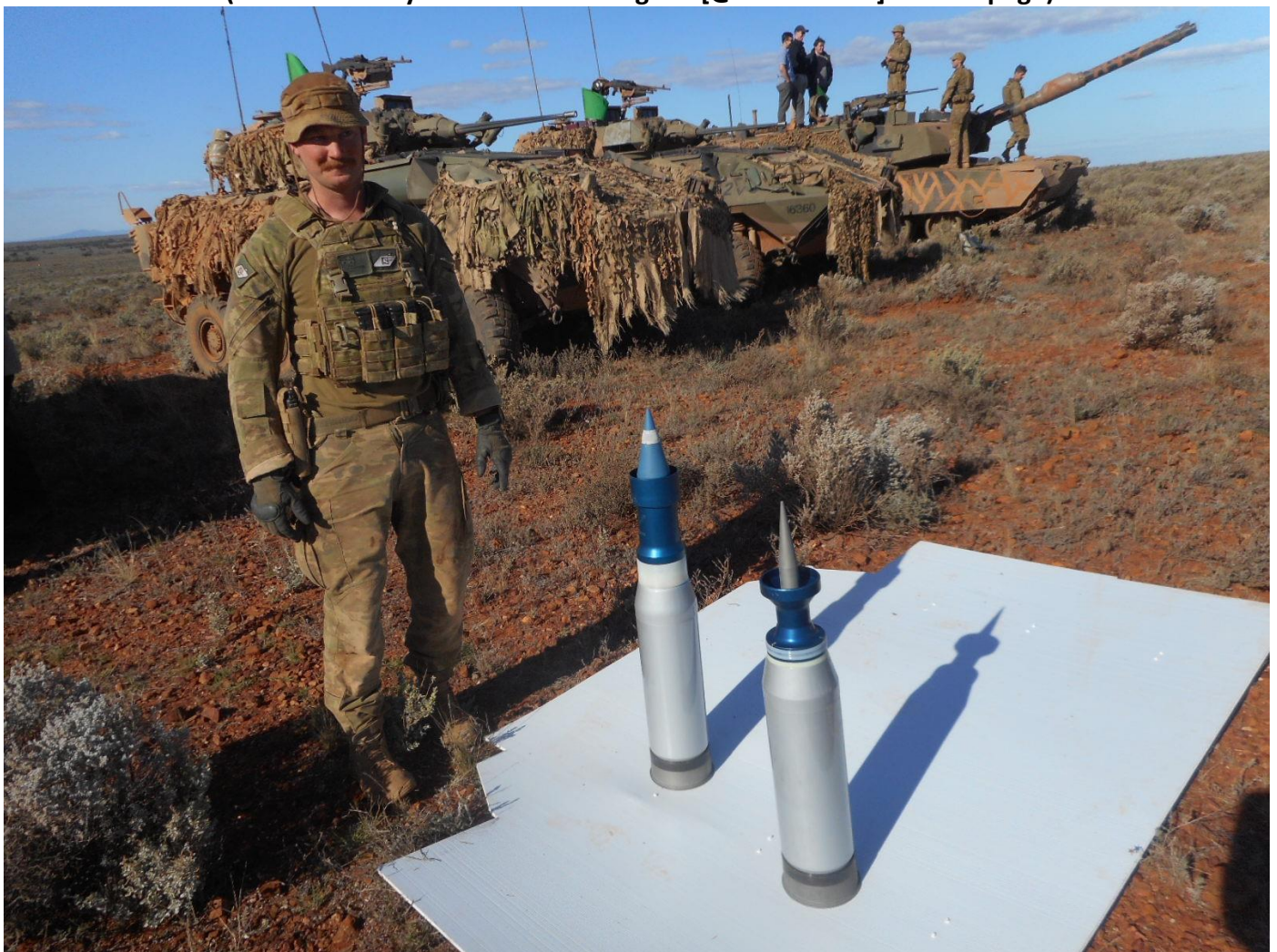
M1A1 Abrams crewman and 120mm practice ammunition on display at the firepower demo M1002 TPMP-T (L) and M865 TPCSDS-T (R) (Photo courtesy Russ Gannon - 1AR Past and Present FB Page)
