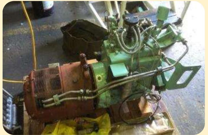
We also struck issues with the water pipes from the radiators to the coolant rails these were close to rusted out we were able to source near new ones from the museum.
